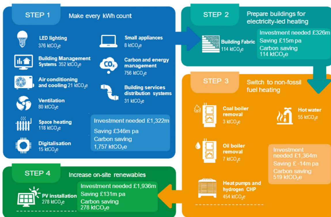
Figure 2.2: Four step approach to decarbonise the NHS estate, Estates 'Net Zero' Carbon Delivery Plan
